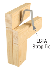
Additional strapping for High Uplift
