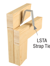
Additional strapping for High Uplift
